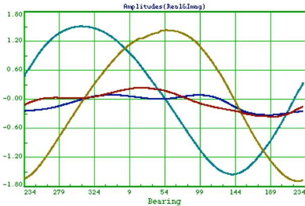
Fig. 3. Real, A13re (red) & A23re (blue), and imaginary, A13im (gold) & A23im (cyan), antenna pattern components
