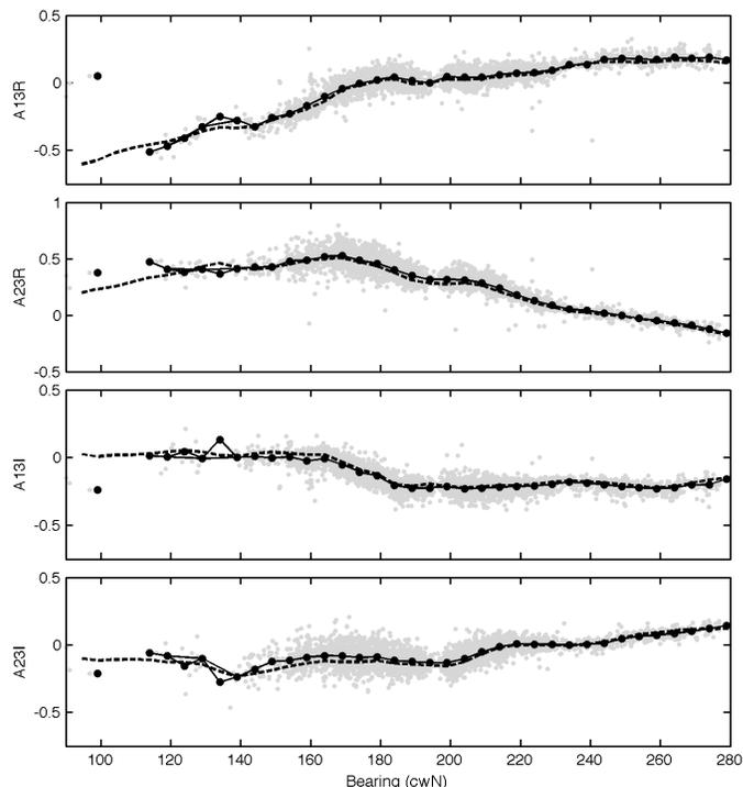
Fig. 5. Normalized antenna pattern measurements from raw vessel echoes with 13 dB IIR filter threshold (gray dots), mean values at  $5^{\circ}$  bins (black dots) and most recent transponder antenna pattern (dotted line).
