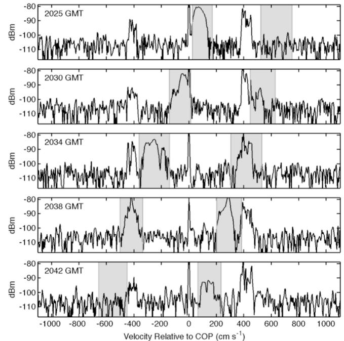
Fig. 4. Five sequential HF radar cross spectra from Coal Oil Point on 6 December 2008. For each plot, the vertical axis shows signal power (dB), and the horizontal axis shows radial velocity (derived from Doppler shifted frequency).
