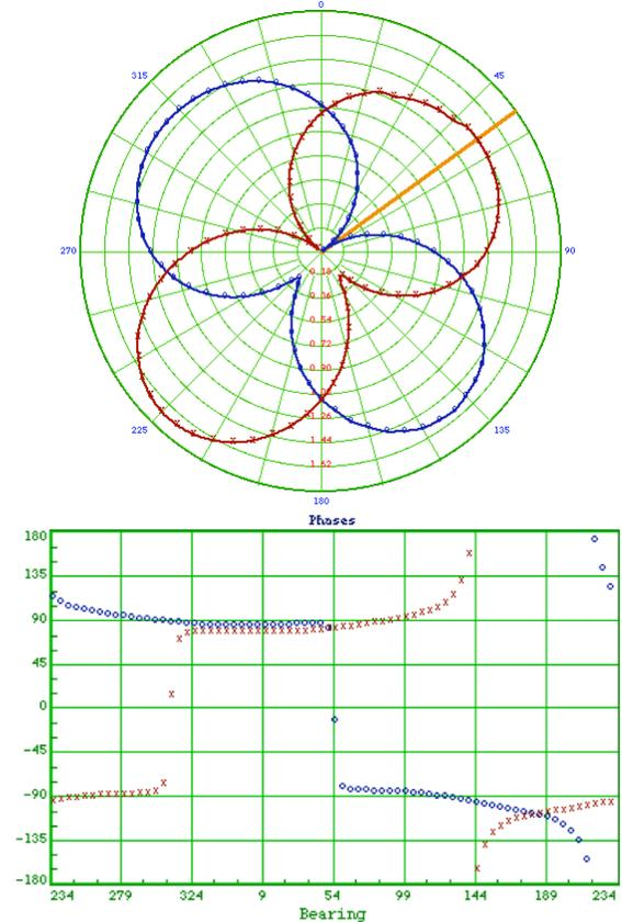
Fig. 2. Example normalized cross-loop amplitude directional pattern (top) and associated phase pattern (bottom) with red and blue plotted for loop 1 and loop 2 normalized values, respectively.
